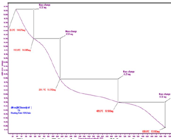
Figure 2. TGA thermogram of Nano-SnO<sub>2</sub>
