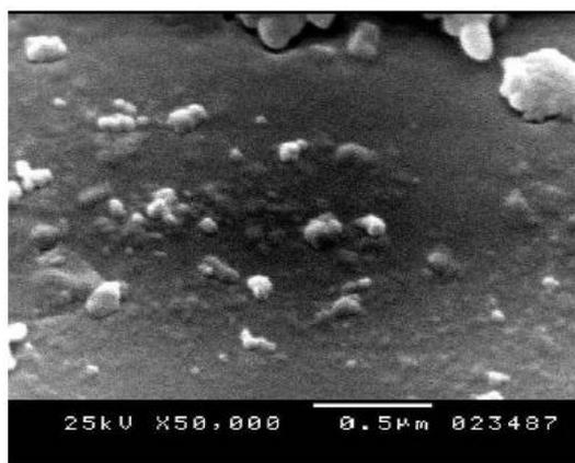
**Figure8.** SEM image of Nano-SnO<sub>2</sub> at magnification order = 50,000x
