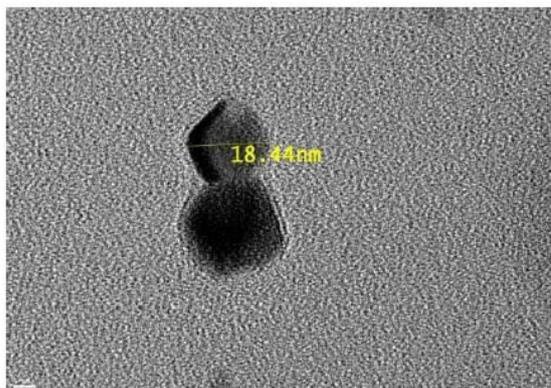
Figure5. Determination of particle size of Nano-SnO<sub>2</sub> by HR-TEM
