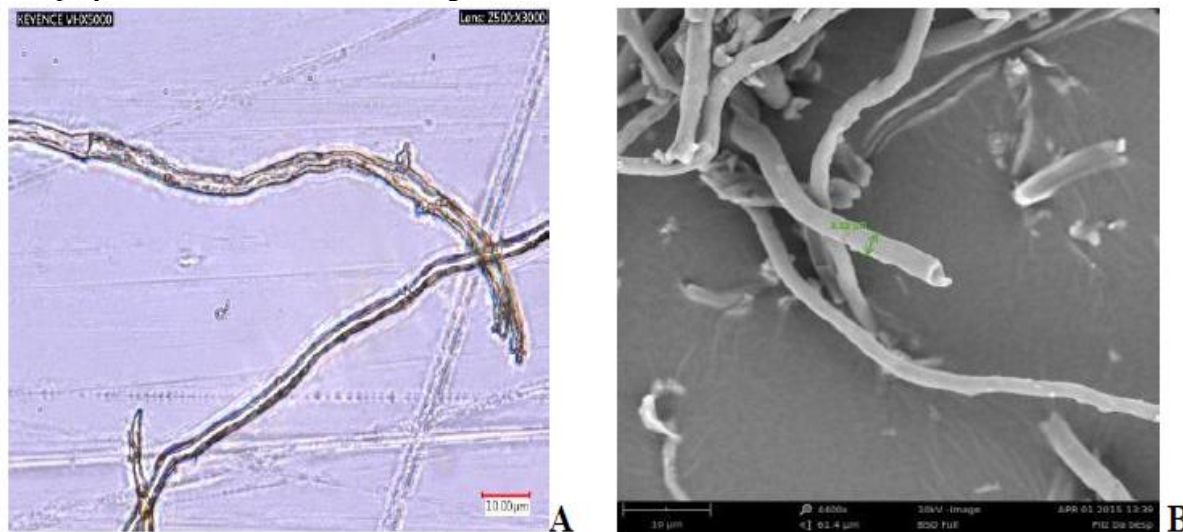
Figure 2. The fibres isolated from tinder fungus fruit bodies. A - Keyence VHX-5000 digital microscope, KEYENCE DEUTSCHLAND GmbH, 3000x. B - The Phenom ProX scanning electron microscope (SEM), LOT-QuantumDesign GmbH, 4400x
