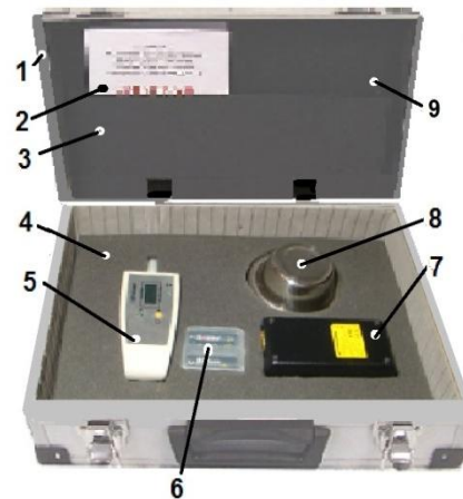
Fig2. DOT: 1-case; 2- Instruction and passport; 3- upper gasket; 4 - lower gasket; 5 - the head of the device; 6 - set of AA batteries; 7 - charger; 8 - cooling table; 9- connecting cables (under item 2).
