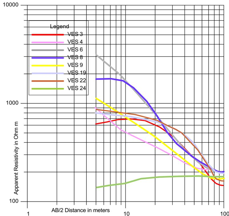
**Figure3.** *VES curves that were interpreted using 2-layer master curves*
