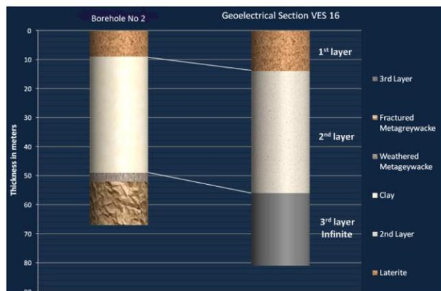
**Figure4.** Correlation of the geo-electrical section with litholog data.
