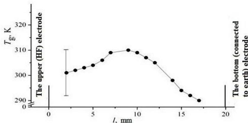
**Fig2.** Distribution of temperature between the electrodes
