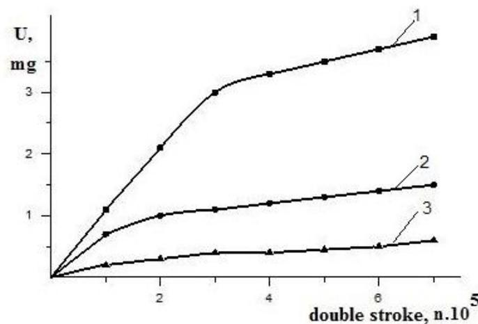
**Fig6.** The wear of standard chromium coatings: 1 – before the treatment; 2 – and after the magnetic pulse effect; 3 – after the plasma effect
