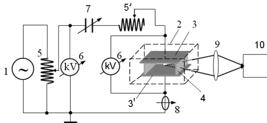
**Fig1.** VCER experimental device: 1 – the generator; 2 – the discharge chamber; 3, 3' – the electrodes of high frequency and ground adapter receptacle; 4 – the quartz window; 5, 5' – the induction windings; 6 – the kilovoltmeter; 7 – the capacitor; 8 – Rogowski-type detector; 9 – the objective; 10 – the spectrometer.
