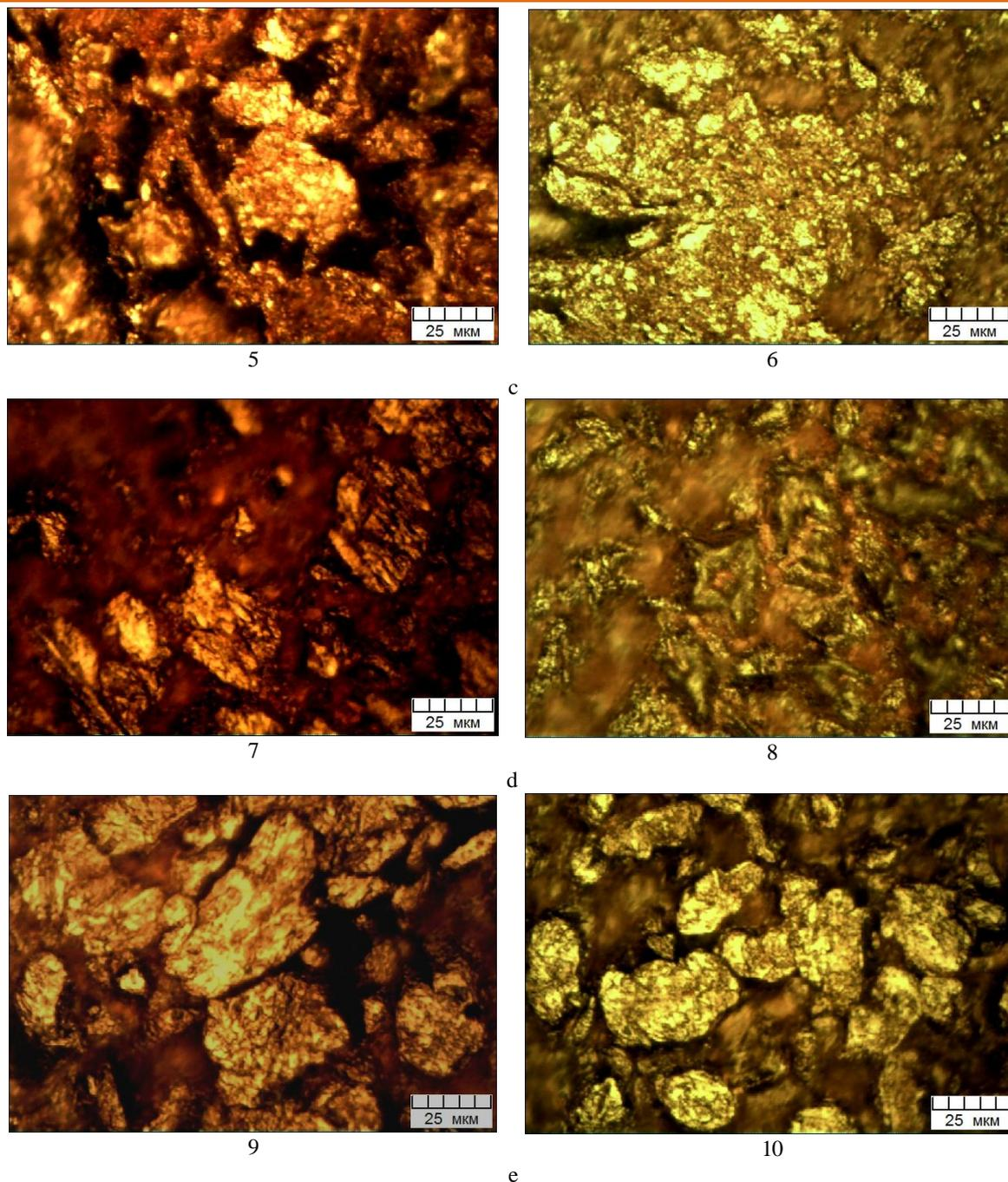
**Fig3.** The morphology of copper coatings (Table 1): 1, 3, 5, 7, 9 – the initial morphology; 2, 4, 6, 8, 10 – the morphology after plasma effect.
