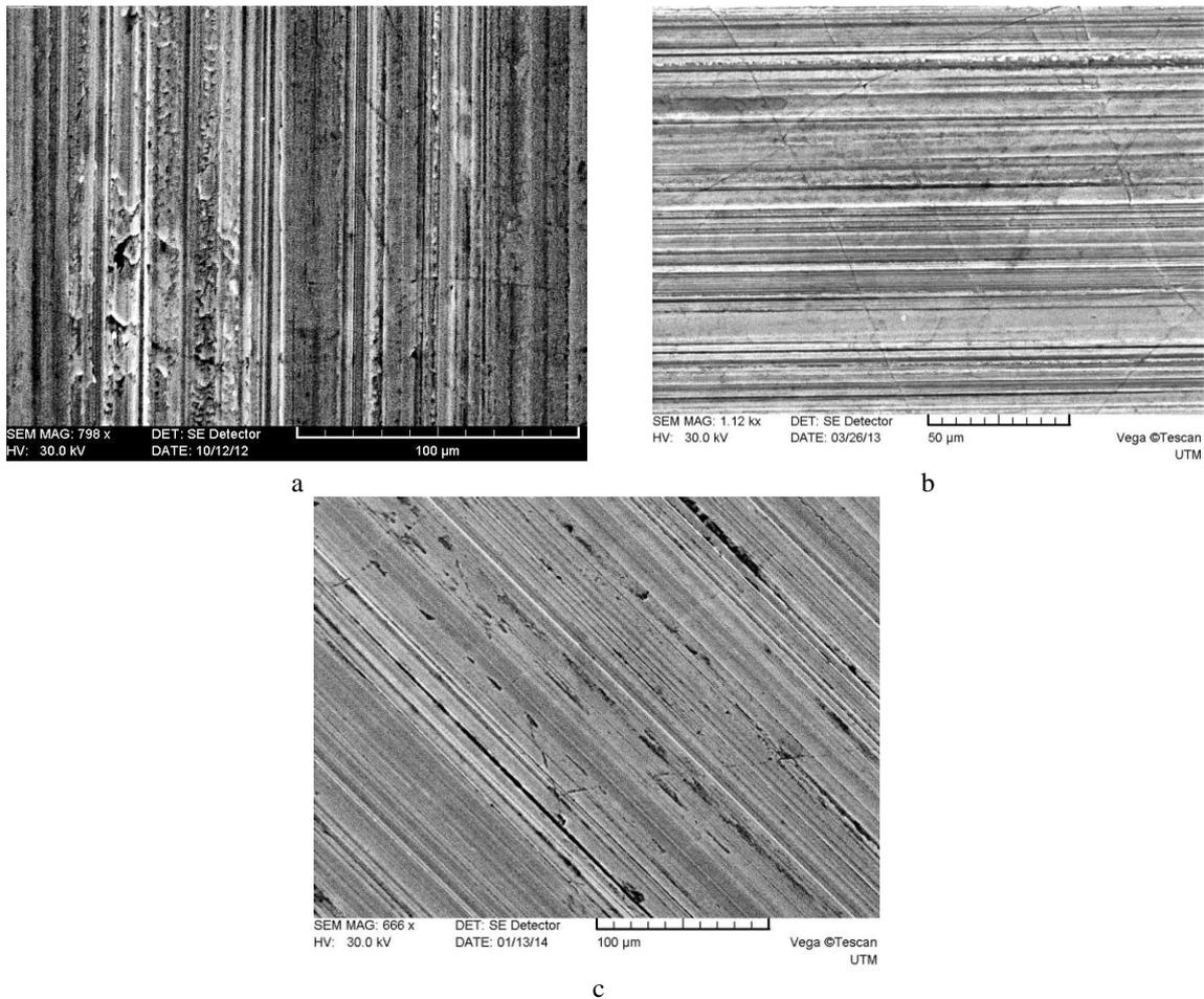
**Fig7.** The worn-out surface of the standard chromium coatings: *a* – before the treatment; *b* – after the magnetic pulse effect; *c* – the same coatings after the plasma effect.
