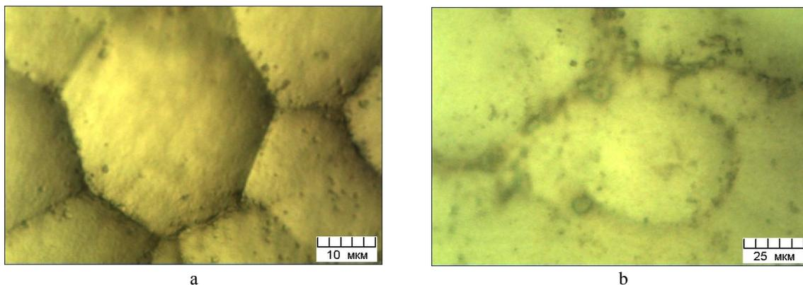
Fig5. The surface morphology of chromium coatings: a – initial, b – after the plasma treatment.
