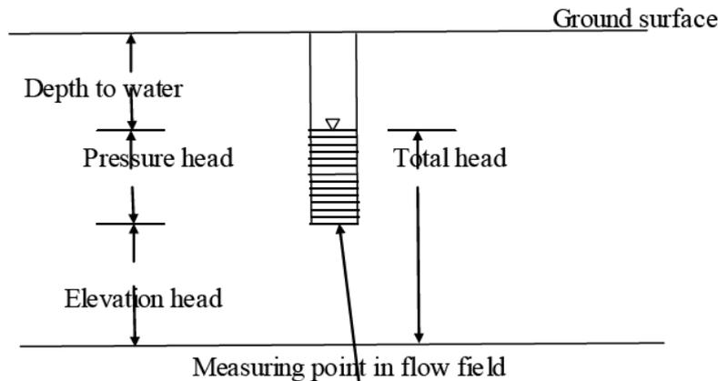
Figure 4. Static water level measurement.
