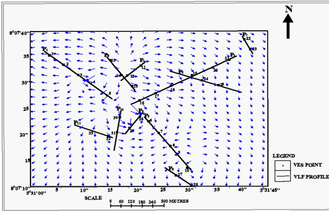
Figure6. Superimposition of groundwater flow direction on the field survey layout.
