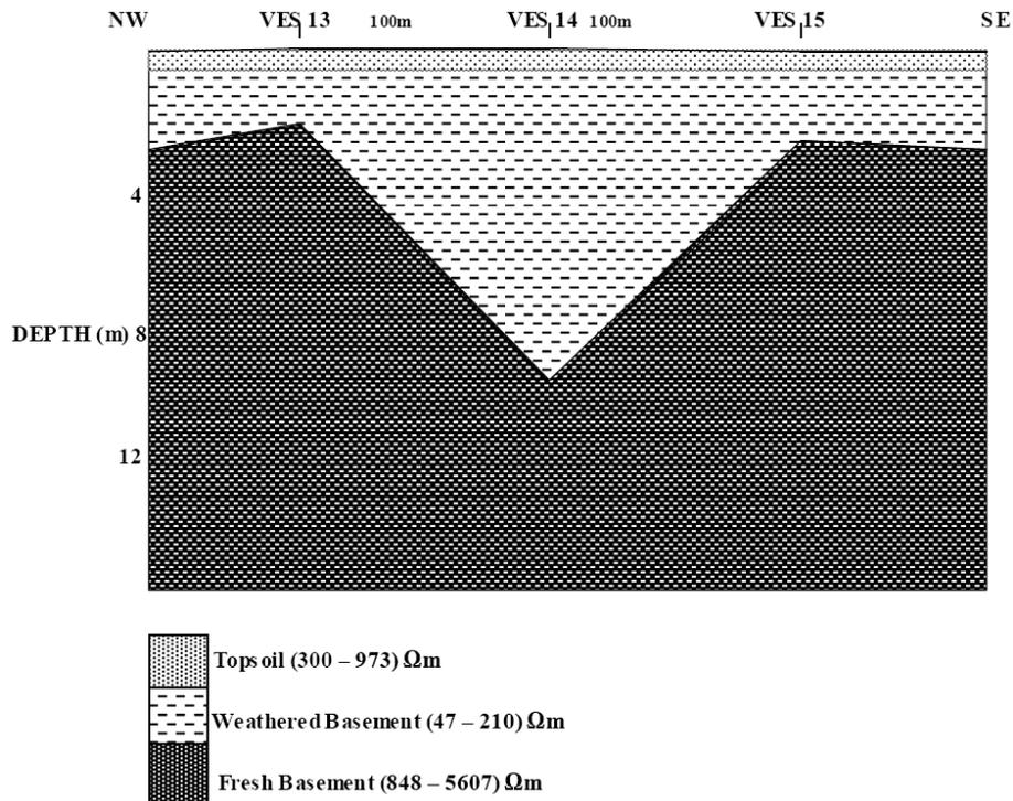
**Figure9.** Representative of Geoelectric section on VLF Profile 5
