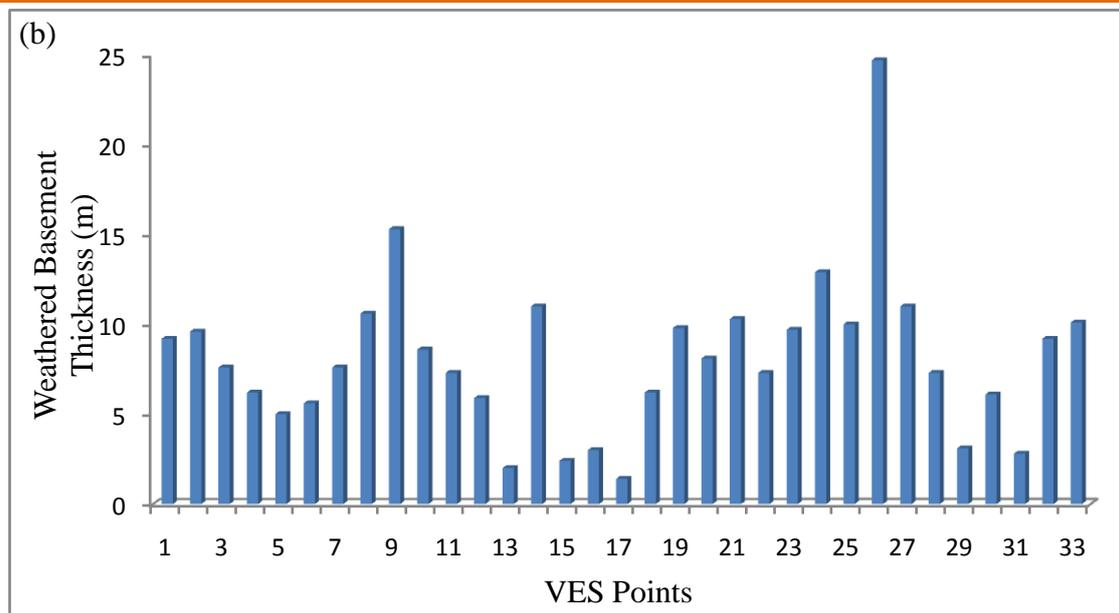
Figure 10. (a) Weathered Basement Resistivity Chart. (b) Weathered Basement Thickness Chart
