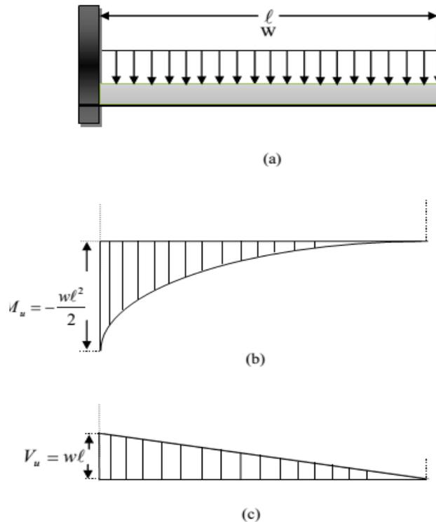
Fig2. The cantilever beam. (a) Uniformly distributed load  $w$ ; (b) moment diagram and (c) shear diagram.
