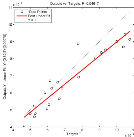
**Fig7.** The scatter plot of the network outputs and targets of the 20 test data for the tension reinforcement ratio  $\rho$  of the radial basis network
