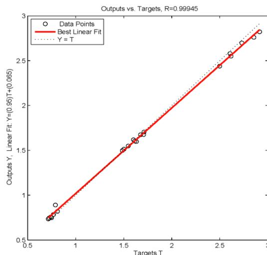
**Fig8.** The scatter plot of the network outputs and targets of the 20 test data for the minimum cost *C* ( $10^3NT$ ) of the radial basis network.
