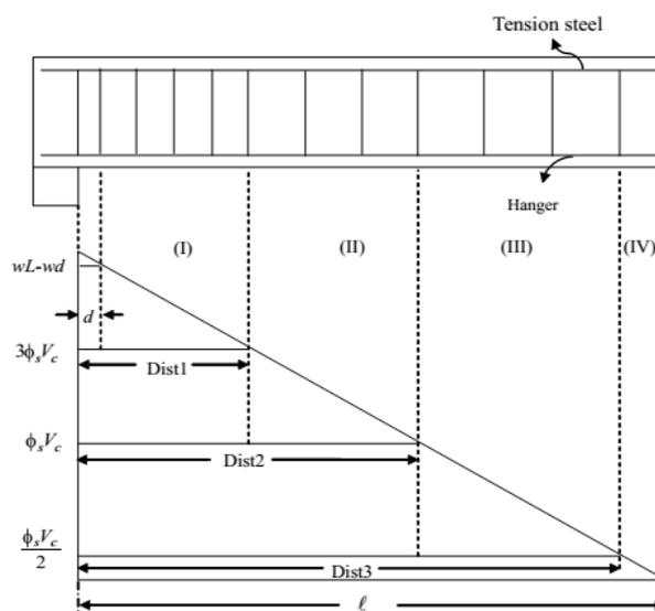
Fig3. Four regions of the cantilever beam to arrange the web reinforcement.
