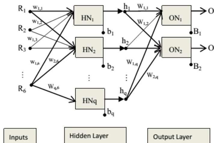
**Fig1.** The feedforward backpropagation neural network with two layers
