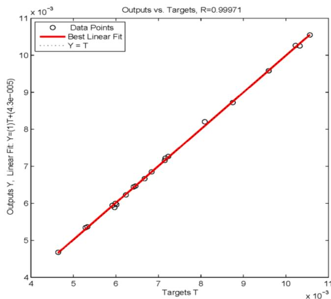
Fig5. The scatter plot of the network outputs and targets of the 20 test data for the tension reinforcement ratio  $\rho$  with 6neurons in the hidden layer.
