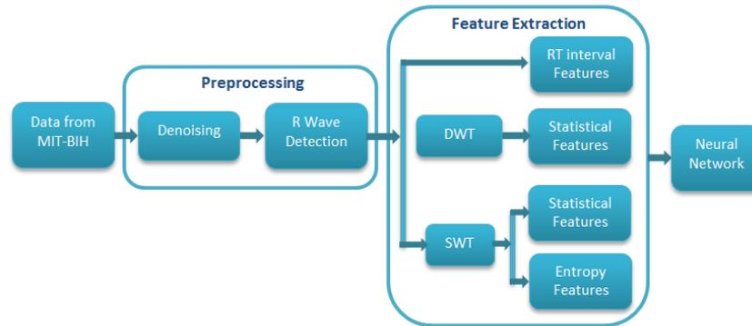
**Fig2.** Block diagram of the ECG beat-classification system
