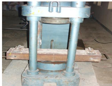
Fig1. Test Setup of CTM with Fixed Roller Base for Shear
