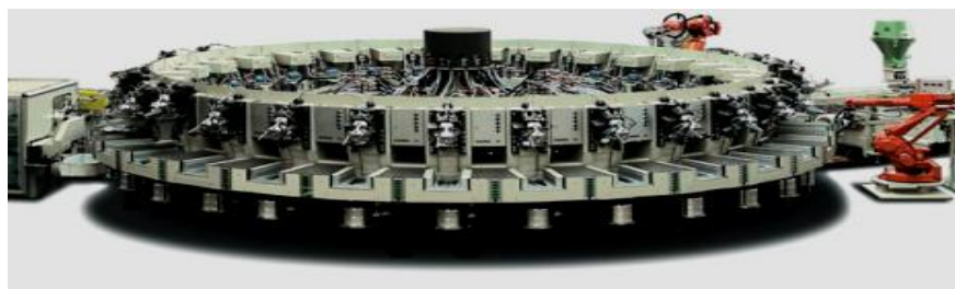
Fig4. Setup of Rotary table with mould bases and robot
