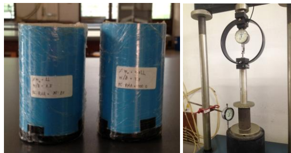
Fig1. Sample prepared and unconfined compression test set up
