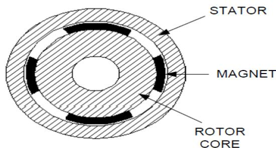
Fig2. Cross section of PMSG.
