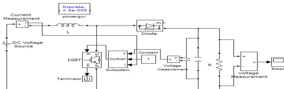
Fig3. Modeling of boost converter
