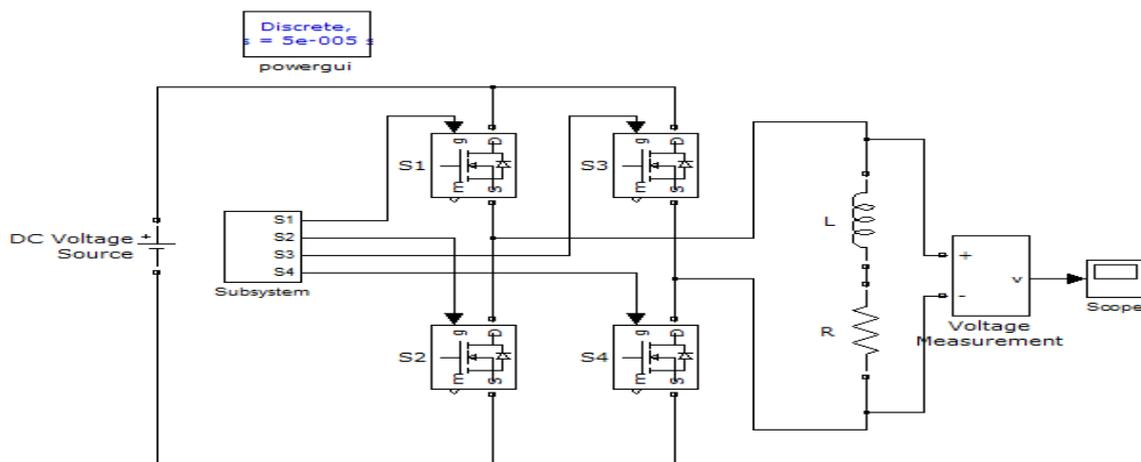
**Fig4.** Modeling of inverter.
