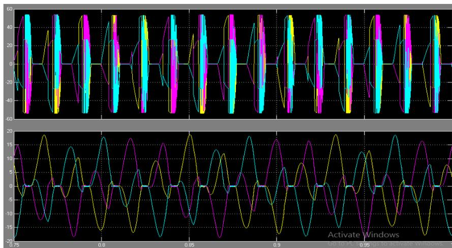
**Fig8.** Generated voltage at wind speed disturbance.
