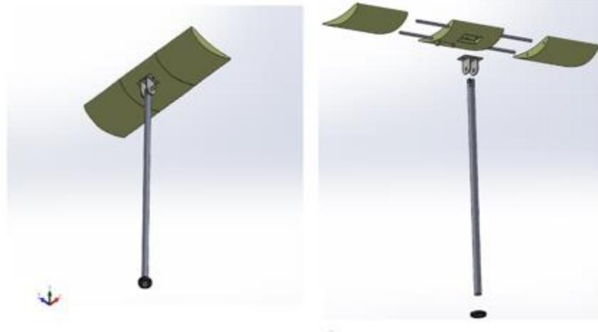
**Figure 4.** General assembly of the wing with rod support.
