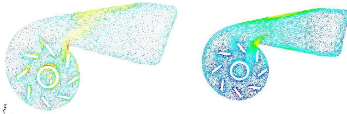
Figure 10. Comparison of velocity vectors of old and new design.
