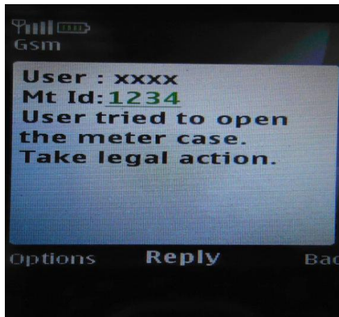
Fig 8. Message Received When User Tried to Open the Meter Case
