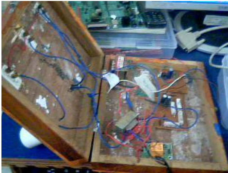
Fig 7. Internal Connections of CT & PT
