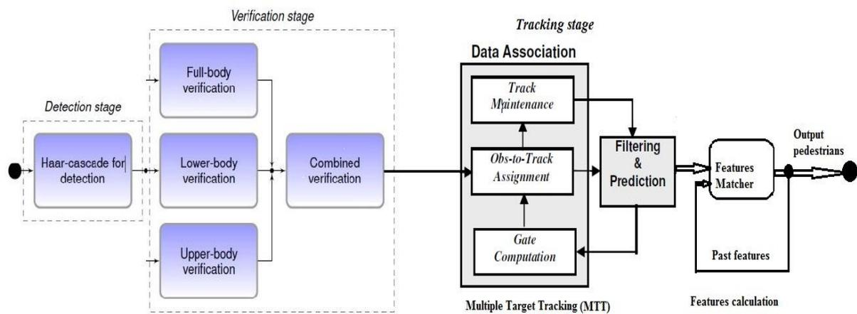
**Fig.2.** System Architectural Diagram for the Proposed PPD.
