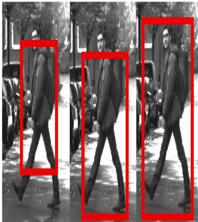
**Fig.3.** Example of the degradation of the bounding box varying  $k$  from 13 in the last pictures to nine in the second picture and to eight in the first picture.
