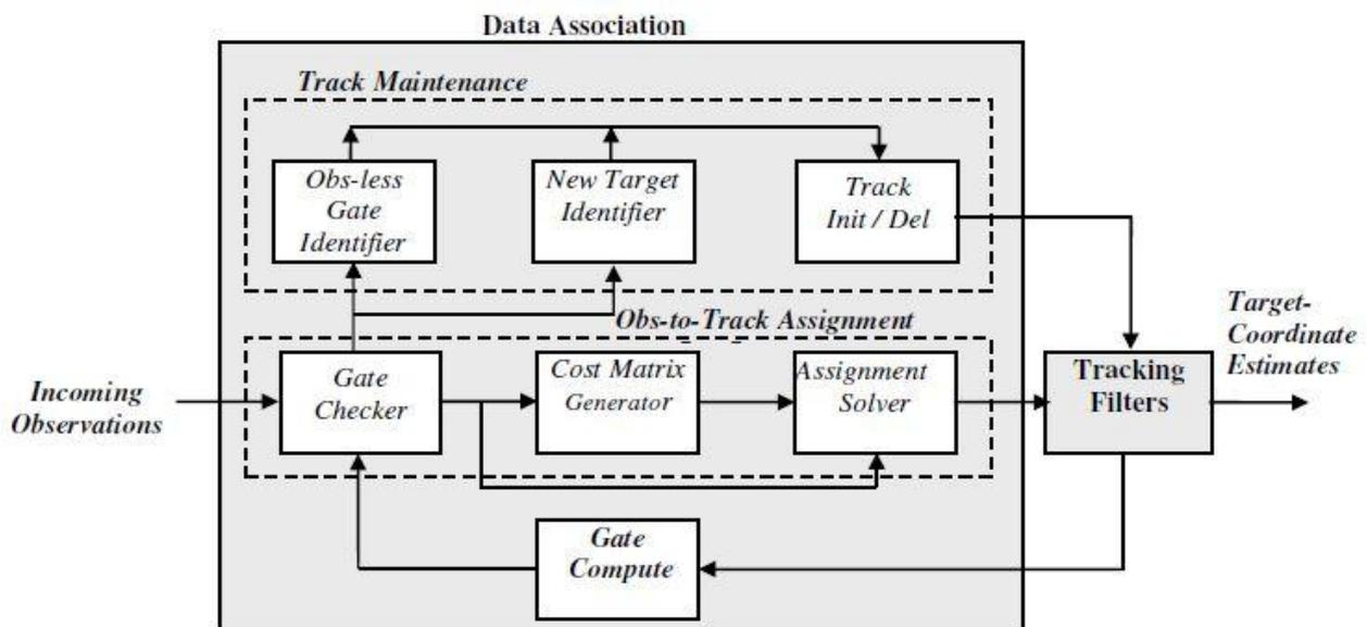
Fig.4. Implementation of Proposed Multiple Target Tracking..
