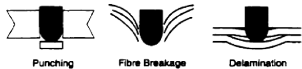
Figure 2. Damage mechanisms occurred in composite materials under ballistic impact [9]
